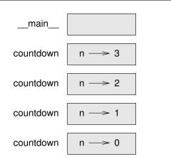
As usual, the top of the stack is the frame for \_\_main\_\_. It is empty because we did not create any variables in \_\_main\_\_ or pass any arguments to it.
