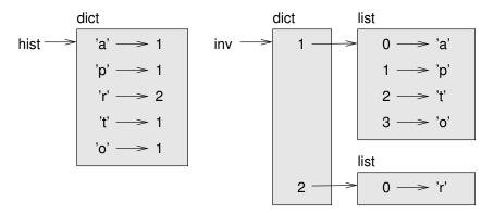
A dictionary is represented as a box with the type dict above it and the key-value pairs inside. If the values are integers, floats or strings, I usually draw them inside the box, but I usually draw lists outside the box, just to keep the diagram simple.
