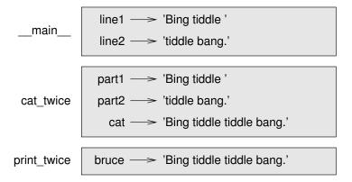
The frames are arranged in a stack that indicates which function called which, and so on. In this example, print\_twice was called by cat\_twice, and cat\_twice was called by \_\_main\_\_, which is a special name for the topmost frame. When you create a variable outside of any function, it belongs to \_\_main\_\_.
