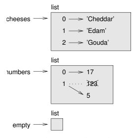
Lists are represented by boxes with the word "list" outside and the elements of the list inside. cheeses refers to a list with three elements indexed 0, 1 and 2. numbers contains two elements; the diagram shows that the value of the second element has been reassigned from 123 to 5. empty refers to a list with no elements.
