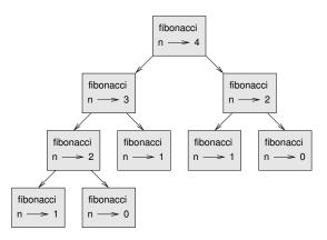
A call graph shows a set function frames, with lines connecting each frame to the frames of the functions it calls. At the top of the graph, fibonacci with n=4 calls fibonacci with n=3 and n=2. In turn, fibonacci with n=3 calls fibonacci with n=2 and n=1. And so on.
